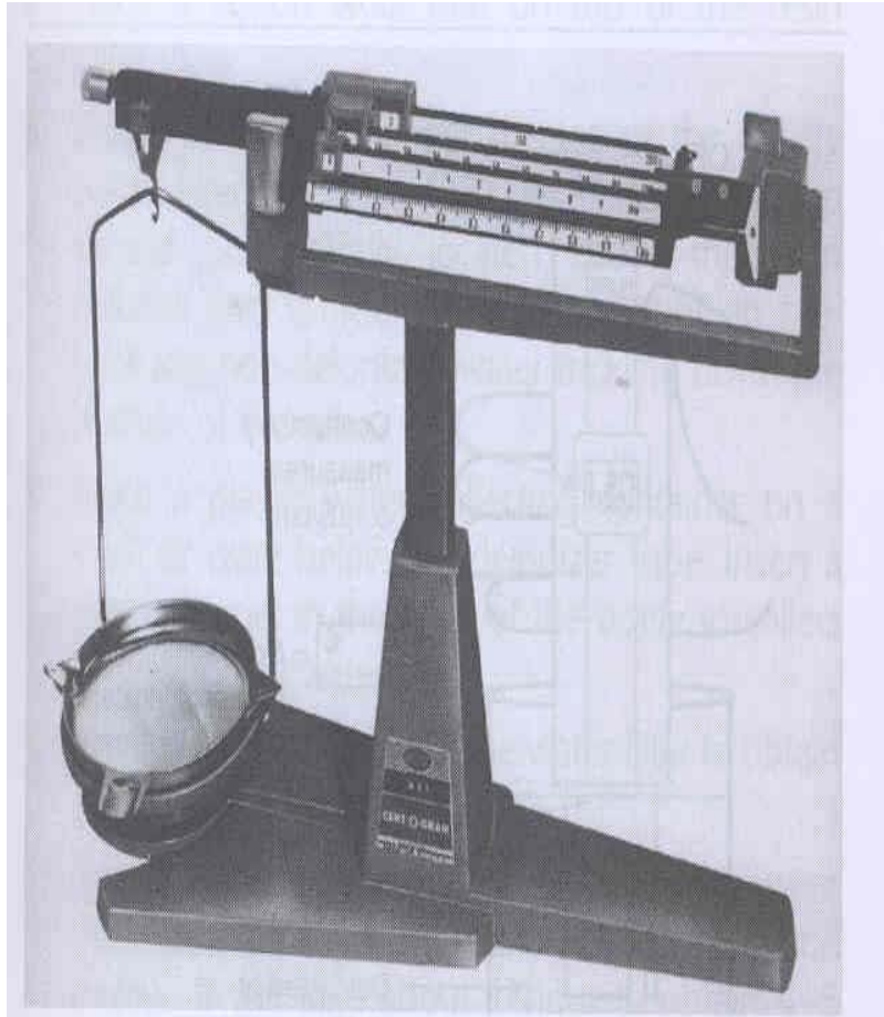
Plate 4.4 Ohaus 311 mechanical beam balance, readability of
