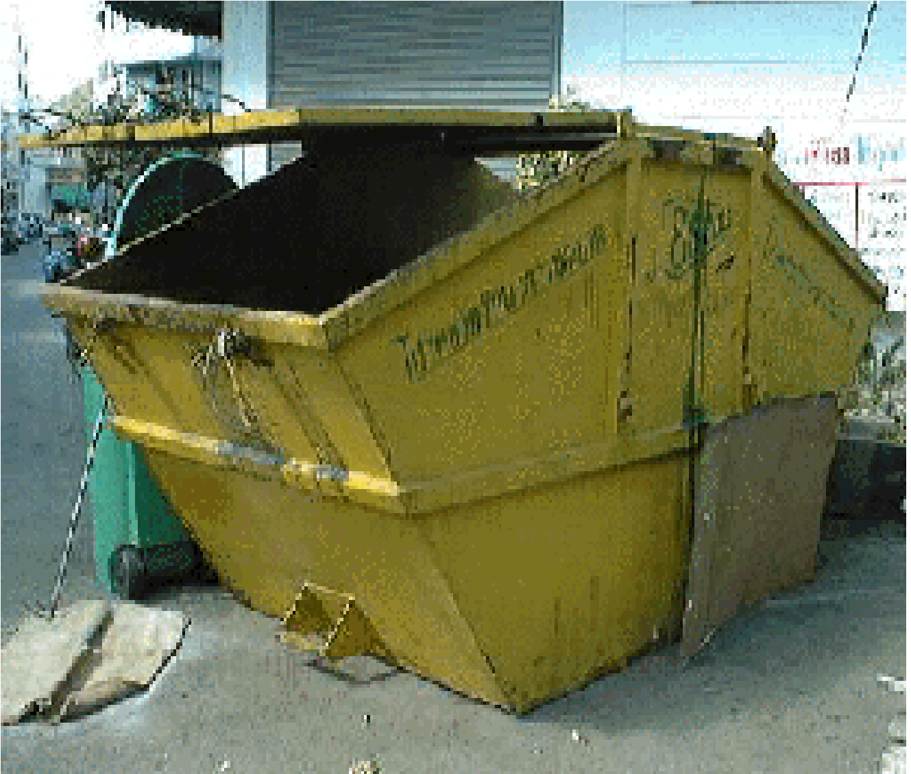
Figure 5-4: Waste containers used in large-volume generator sites.
