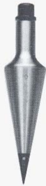
Fig. 4.4. A plumb bob: (is one of the simplest yet most important accessories for accurate surveying.)
